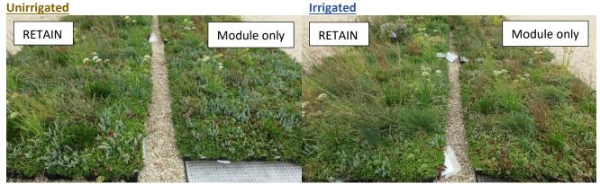
**Standard module system.** Left panel is unirrigated. RETAIN showed 1% increase in sedums and 78% increase in non-sedums. Right panel is irrigated. RETAIN showed 12% decrease in sedums and 37% increase in non-sedums.
