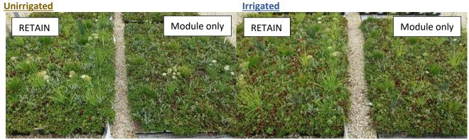
**Lite module system**. Left panel is unirrigated. RETAIN showed 57% increase in sedums and 50% increase in non-sedums. Right panel is irrigated. RETAIN showed a 42% increase in sedums and 101% increase in non-sedums.
